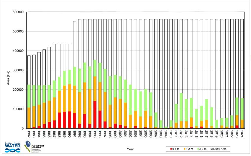
The Shepparton Irrigation Region Watertable Contours map (on reverse page) was produced using information from 1,000 groundwater level monitoring bores. The graph shows the total study area and a comparison of the areas of watertable at various depths from 1982 to 2024. High watertables (less than two metres below surface) and their associated salinity issues will remain a significant risk except in times of extended drought.
